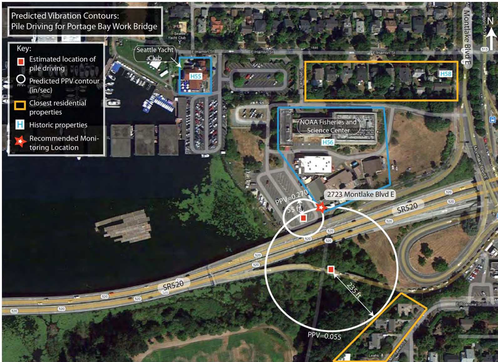
Figure 7-10: Predicted Vibration Contours for Portage Bay Bridge Pile Driving, East End
