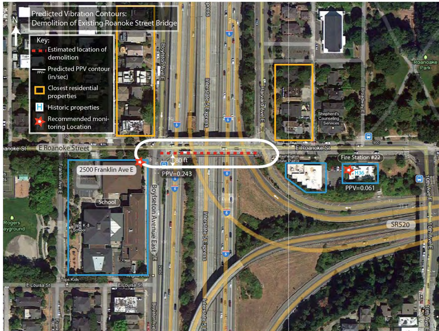
Figure 7-12: Predicted Vibration Contours for Limited Demolition of Existing Roanoke Street Bridge, I-5 Interchange Area
