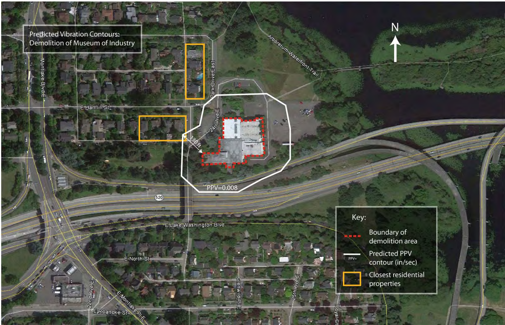
Figure 7-7: Predicted Vibration Contours for Demolition of Museum of History and Industry (MOHAI)
