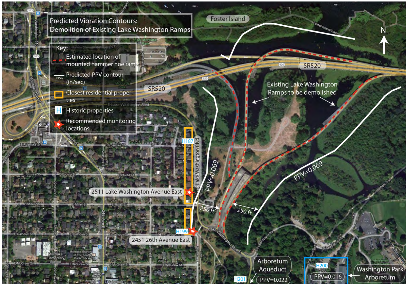
Figure 7-4: Predicted Vibration Contours for Demolition of Existing Lake Washington Ramps in West Approach Area
