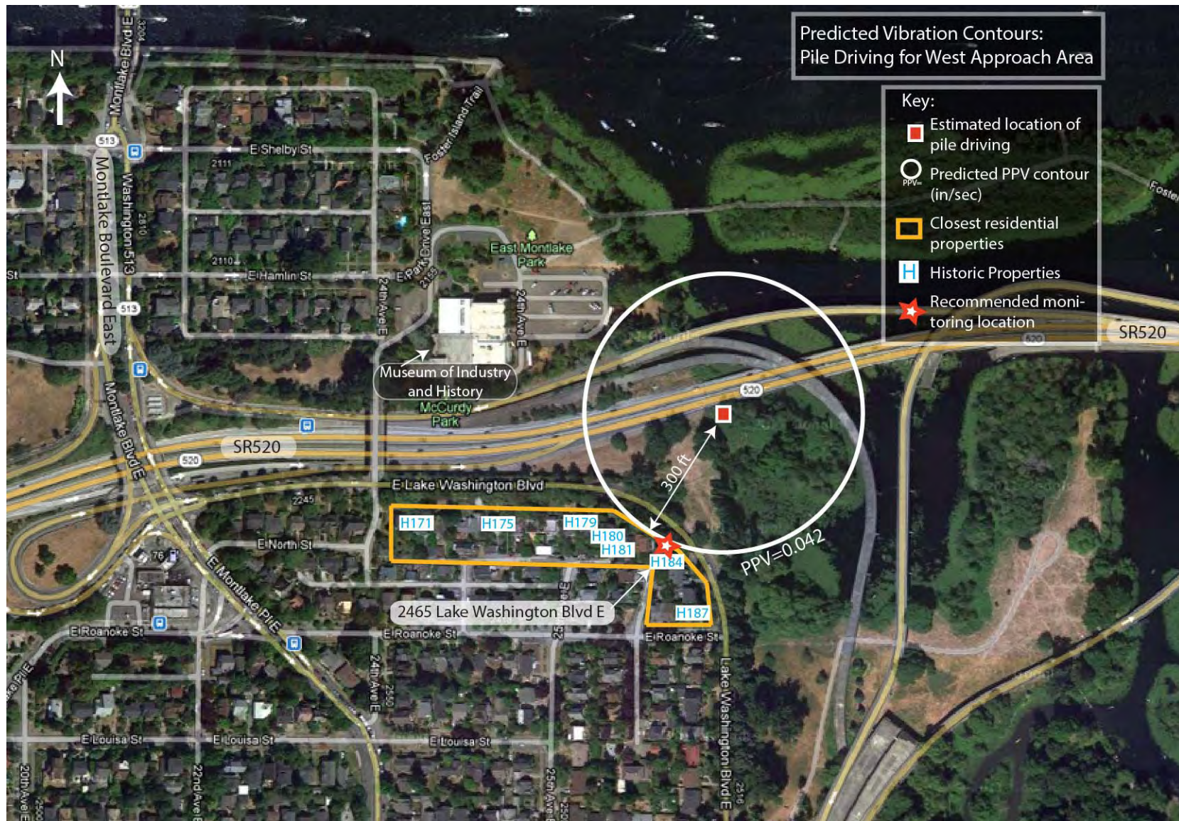
Figure 7-1: Predicted Vibration Contours for West Approach Pile Driving, West End
