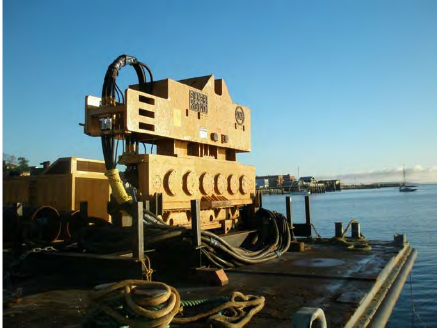
Figure 3. APE Super Kong 600 vibratory hammer.
