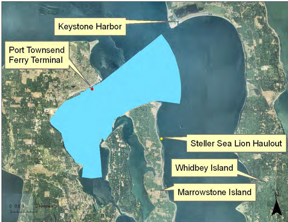
Figure 21. Approximate extent of in-water noise for Port Townsend Test Pile Project vibratory pile driving with 6800 meter attenuation to 120 dB RMS.
